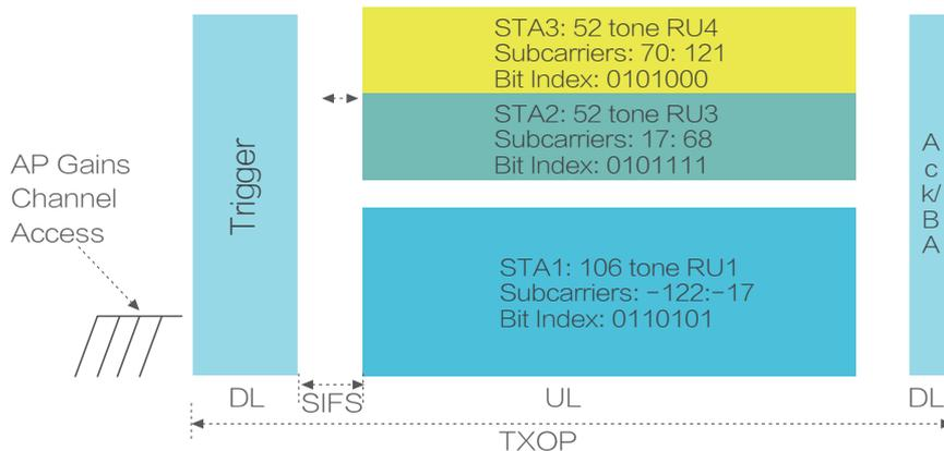
As shown in the preceding figure, the AP sends a trigger packet to allocate RUs to three STAs. The STAs jointly send HE TB packets after one SIFS. The AP returns an ACK or a BA after receiving the HE TB packet.
