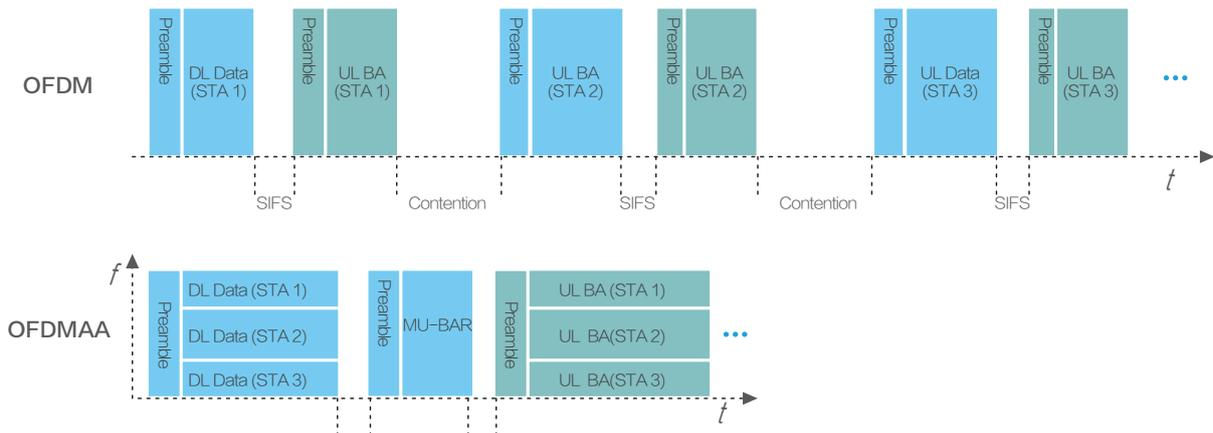
As shown in the preceding figure, OFDMA reduces preambles, interframe spaces such as short interframe spaces (SIFs), and contention backoff time of STAs, thereby increasing communication efficiency in concurrency scenarios.
