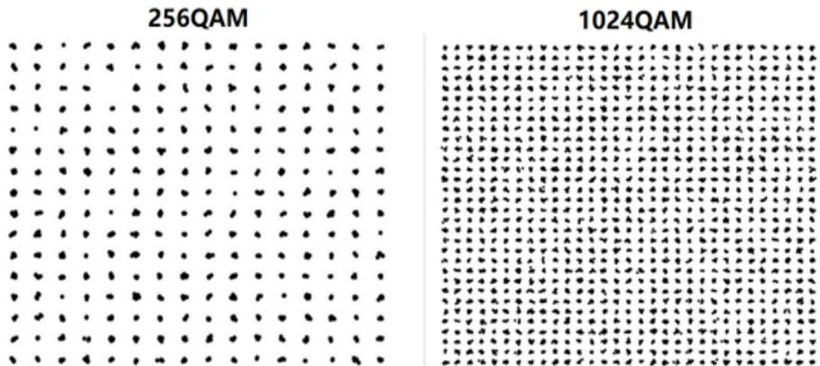
Due to the increase in the information density of 1024QAM, the difference between signals carrying different codes is also smaller, and the requirements for signal quality are also higher. Therefore, the technology can only fully exert its advantages in a scenario with excellent wireless environment and relatively close distance, such as small office and conference room with good signal.
