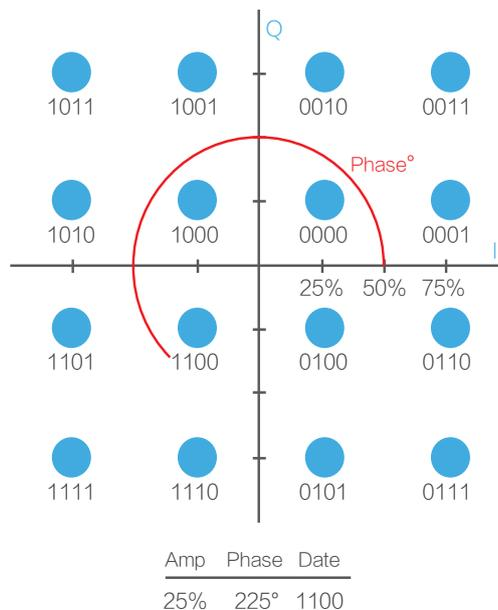
A maximum of 256QAM is supported in the 11ac era. 11ax introduces a higher-order coding, 1024QAM. A signal unit of 1024QAM represents 10 bits (1024 types) of data, which offers 25% higher performance than 256QAM.
