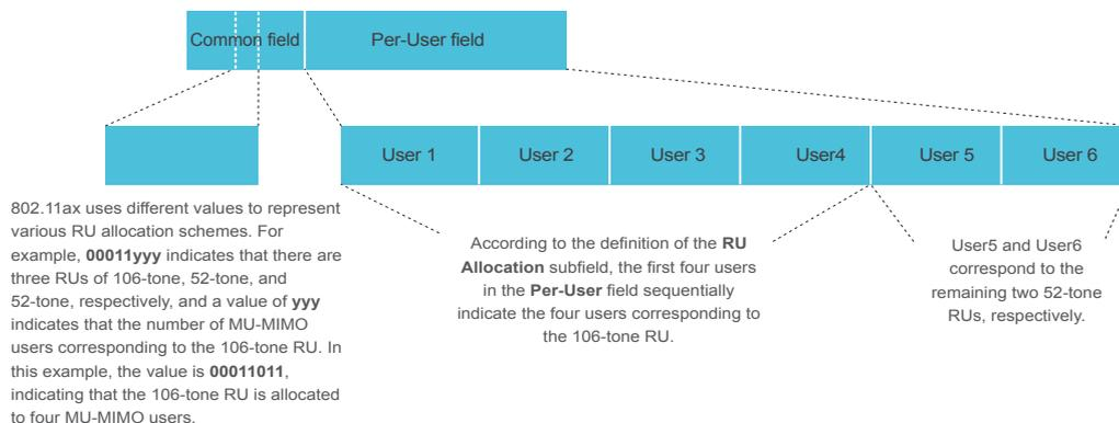
802.11ax gives free rein to form various combinations of OFDMA and MU-MIMO, and can alternatively enable OFDMA transmission and MU-MIMO transmission separately. Combinations of OFDMA and MU-MIMO are not supported until 802.11ax Wave 2 due to its complexity.
