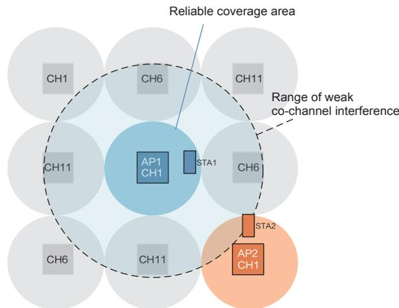
Wi-Fi protocols before 802.11ax all use the clear channel assessment (CCA) threshold to determine whether a channel is busy, thereby determining whether packets can be sent. 802.11 protocols define the following thresholds:
