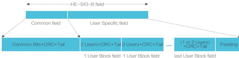
The HE-SIG-B field has a variable length, and consists of the Common field and User Specific field.
