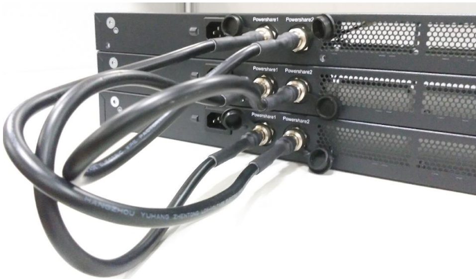
Figure 3-12 Connecting Cables Among Three Switches 3
