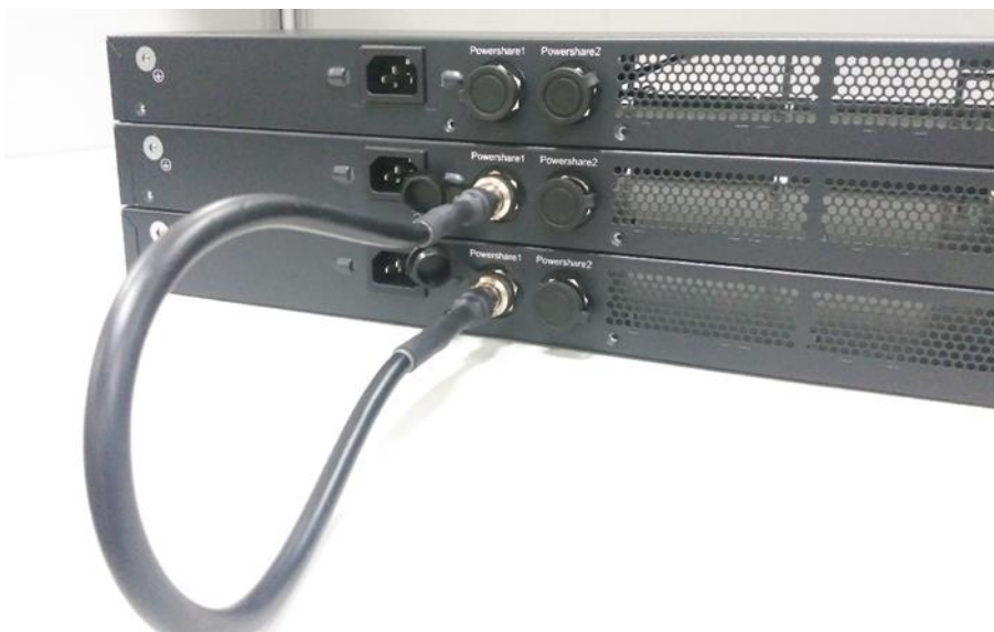
Figure 3-11 Connecting Cables Among Three Switches 2
