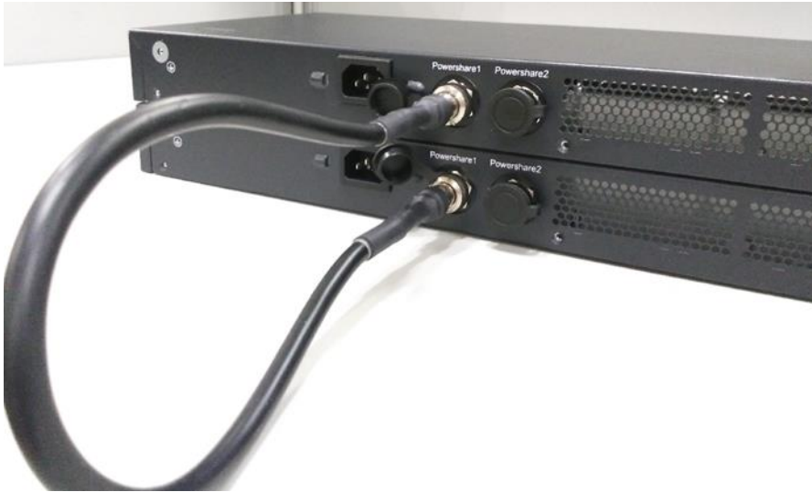
Figure 3-9 Connecting Cables between Two Switches
